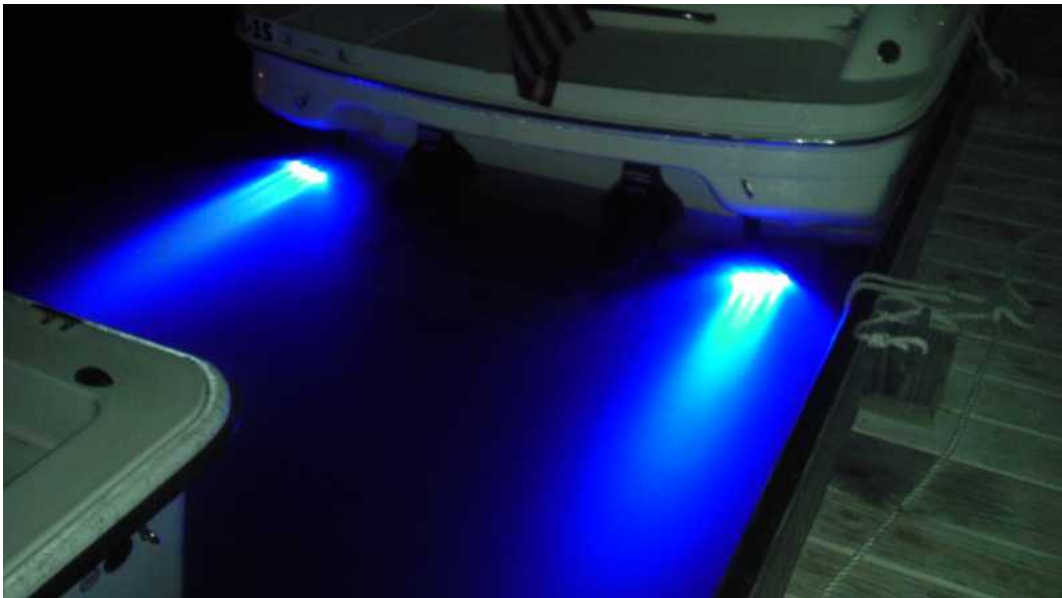
Four blue spotlights mounted on the trim tabs
